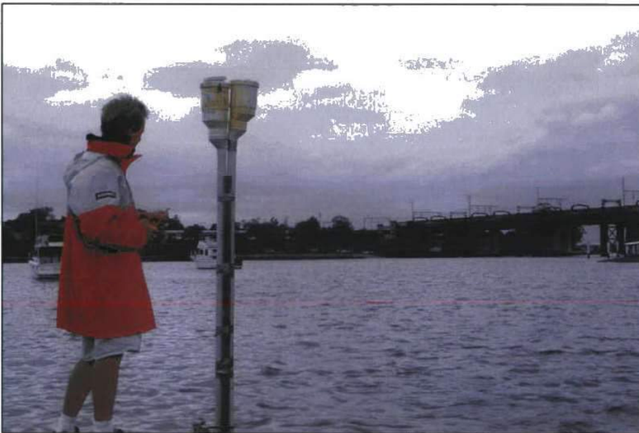
■ Figure 2-4 Tide gauge at John Whitton Bridge
